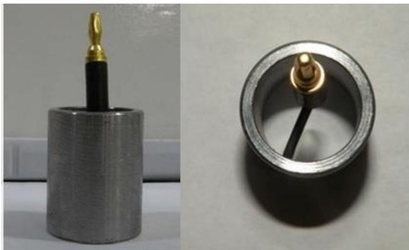
Figure 29: Specimen for HPHT rotating cylinder electrode
